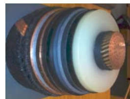
Ormen Lange 420 kV/1000MW 1x1200 mm 2 Cu
