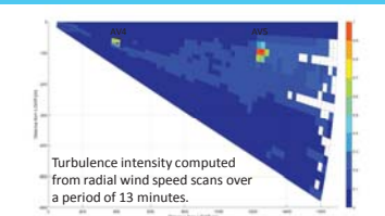
Example of Plan Position Indicator (left column) and Range Height Indicator (right column) scan scenarios directed towards the AV 4 and AV5 wind turbines (denoted by the red dots).
