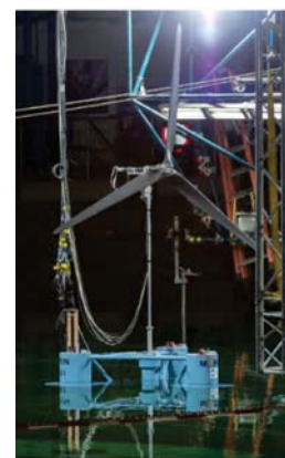
Instrumented OC5-DeepCwind model in the MARIN offshore basin
