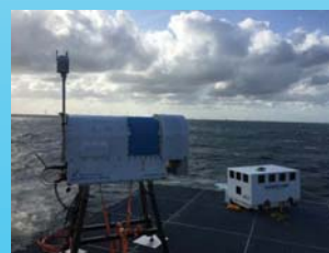
Passive microwave radiometer deployed at FINO1, next to a WindCube V1.
