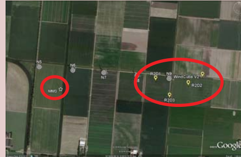
Layout of the test site with turbine, mast and LiDARs indicated.
