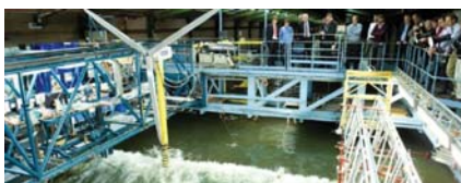
Breaking wave on monopile foundation from MARINs WiFi model test campaign
