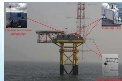
Meteorological OBLO instrumentation deployed at the German research platform FINO1 in the North Sea.
