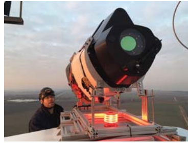
Nacelle LiDAR installation
