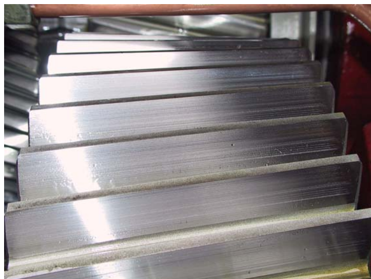
Figure 3 Criteria and picture for Gearbox, Tooth – Micropitting, State 1:
