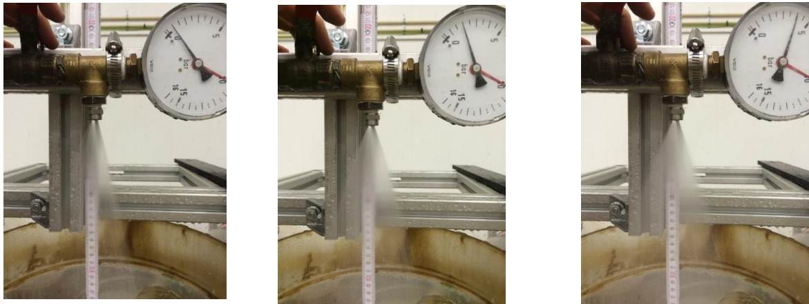
Water jets from nozzle JBF 2124 B1 at 1, 2, and 4 bars.
