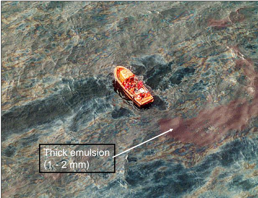
Figure A-12: Surface oil slick (initial thickness > 200 \mu\text{m} ) from the experimental deep-water release "DeepSpill" in 2000. Surface oil is emulsifying similar to an oil slick from a surface batch release (from Leirvik et al., 2011)
