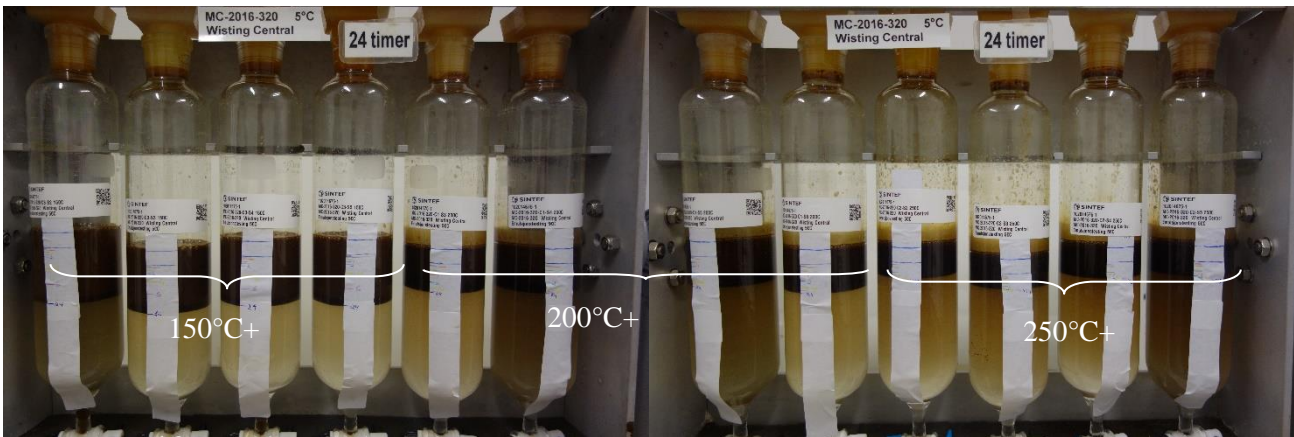
Figure 2-3: The rotating cylinders at the start and after 24 hours of rotation at 5 °C
