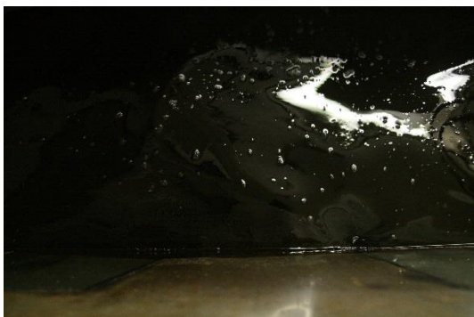
Sample 0 (start): The crude oil is black and was easily distributed on the water surface.
