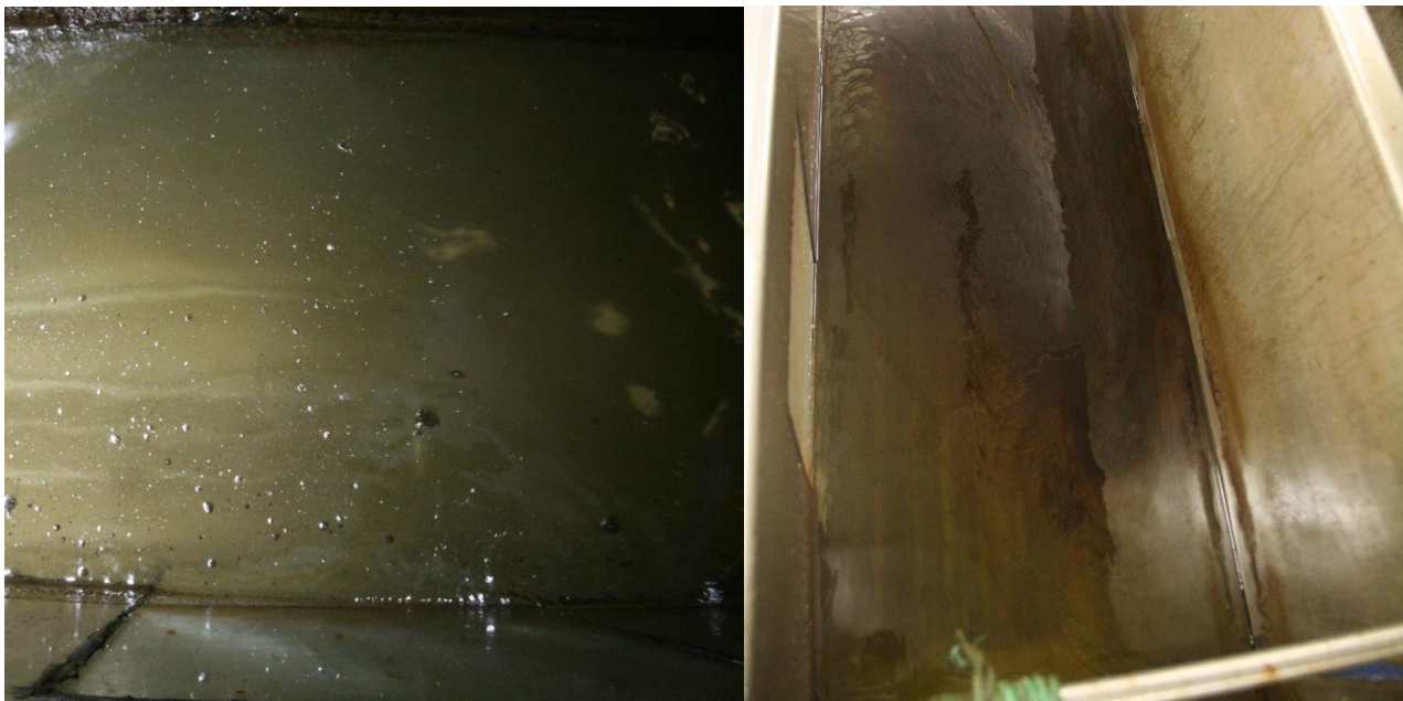
Left: Sample 7 (24 hours): No change visually changes from 12 hours weathering. Right: Sample 8 (48 hours): The wave action was turned off and the oil/emulsion was collected. Estimated oil/emulsion: ~50 mL.
