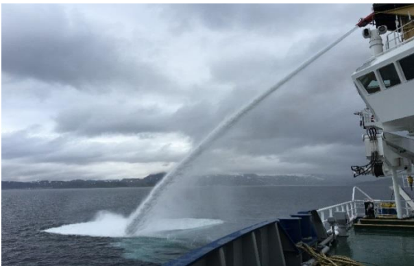
Figure 5-7 Pre-testing of Fi-Fi-monitors (left) and high-capacity water-flow boom on MS Strilborg at Hammerfest, May 23-25, 2016). Part of the "Oljevern 2015 program "Mechanical Dispersion of Thin oil films" funded by NOFO.
