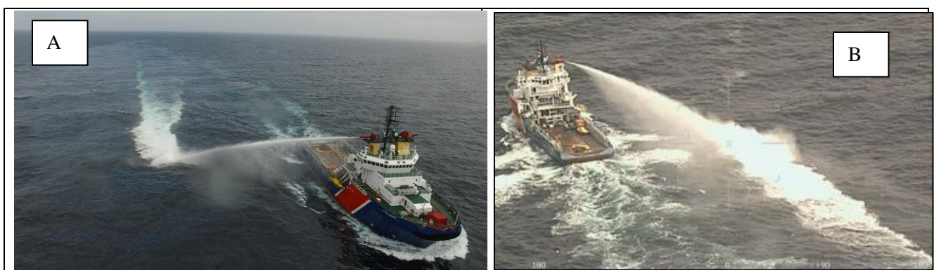
Figure 7-25 Water flushing using SB Fi-Fi monitor on MS Strilborg. Drone video by Maritime Robotics (A) and ©Finnish Border Guard / SYKE (B).
