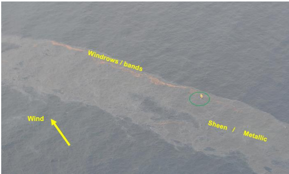
Figure 7-24 Bands of loose emulsion (1-2 mm thick) surrounded by a thin oil film of primarily "Sheen" and "Metallic" (i.e. < 50 micron, BAOAC) in experiment TOF 3.3 (13:14 LT), (©Finnish Border Guard / SYKE).
