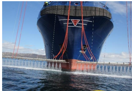
Figure 5-7 Pre-testing of Fi-Fi-monitors (left) and high-capacity water-flow boom on MS Strilborg at Hammerfest, May 23-25, 2016). Part of the "Oljevern 2015 program "Mechanical Dispersion of Thin oil films" funded by NOFO.
