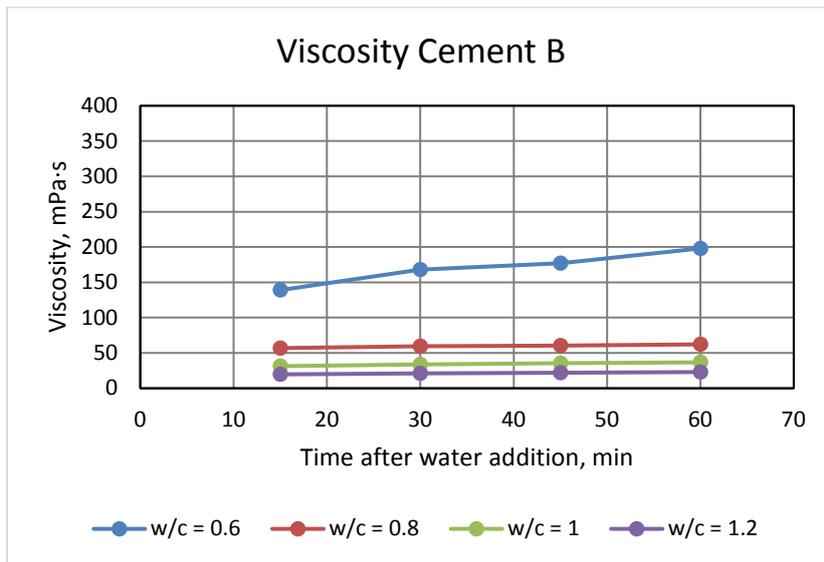
**Figure 9** Viscosity development for Cement B
