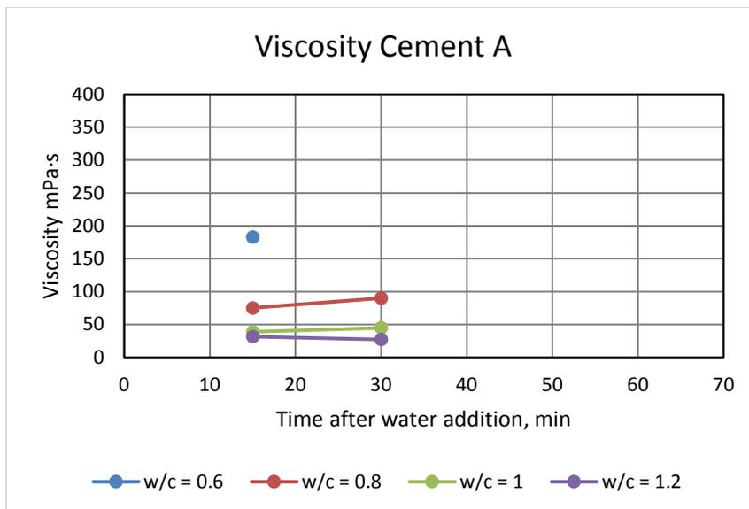
**Figure 8** Viscosity development for Cement A
