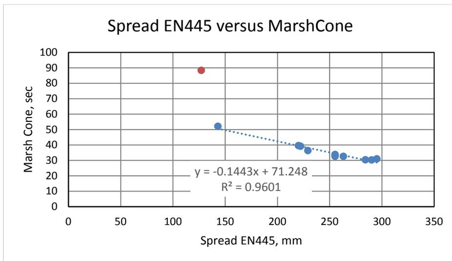
**Figure 5** Relation between spread according to EN445 and Mars Cone test results at 20°C. The red point represents Cement B at w/c = 0.6 (w/c = 0.6 for cement C did not give any Marsh Cone result)
