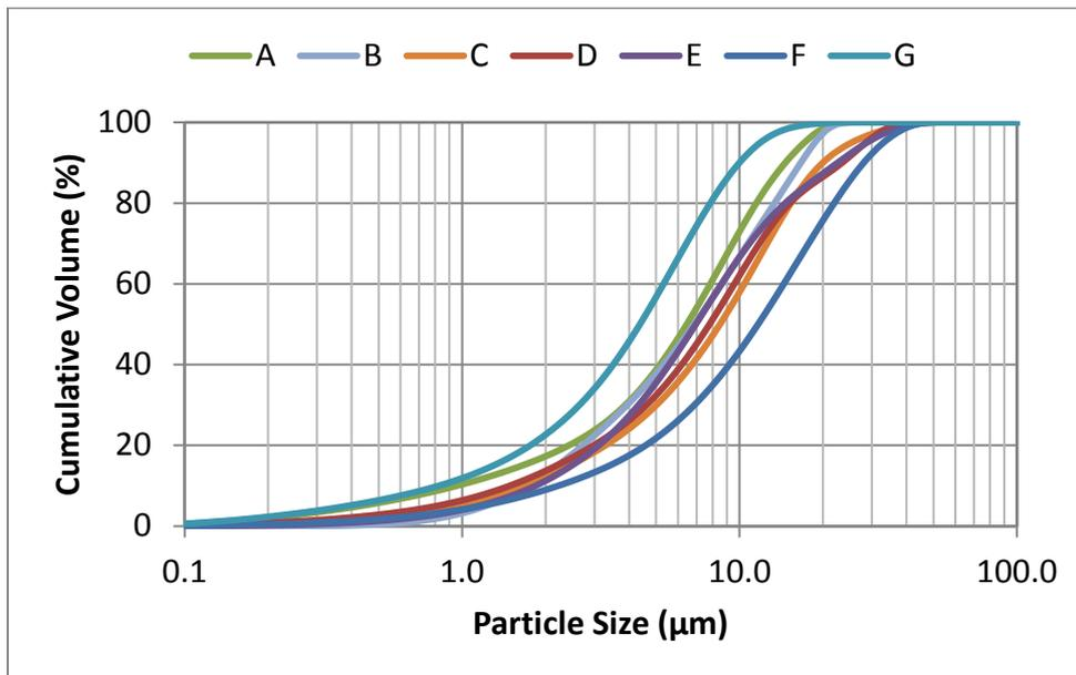
**Figure 1 Particle size distribution for tested cements**
