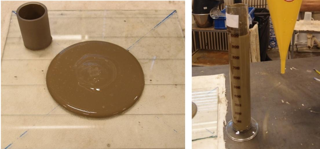
**Figure 4** Spread EN445 (left) and Marsh Cone with 1 litre graduated cylinder (right)
