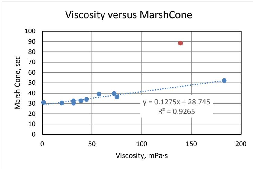
**Figure 7** Viscosity after 15 min versus Marsh Cone values. The red spot is  $w/c = 0.6$  for cement B ( $w/c = 0.6$  for cement C did not give any Marsh Cone result)
