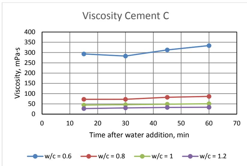
**Figure 10** Viscosity development for Cement C
