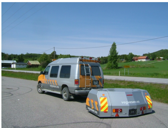
Figur 2.1 CPX-tilhenger, Statens vegvesen
