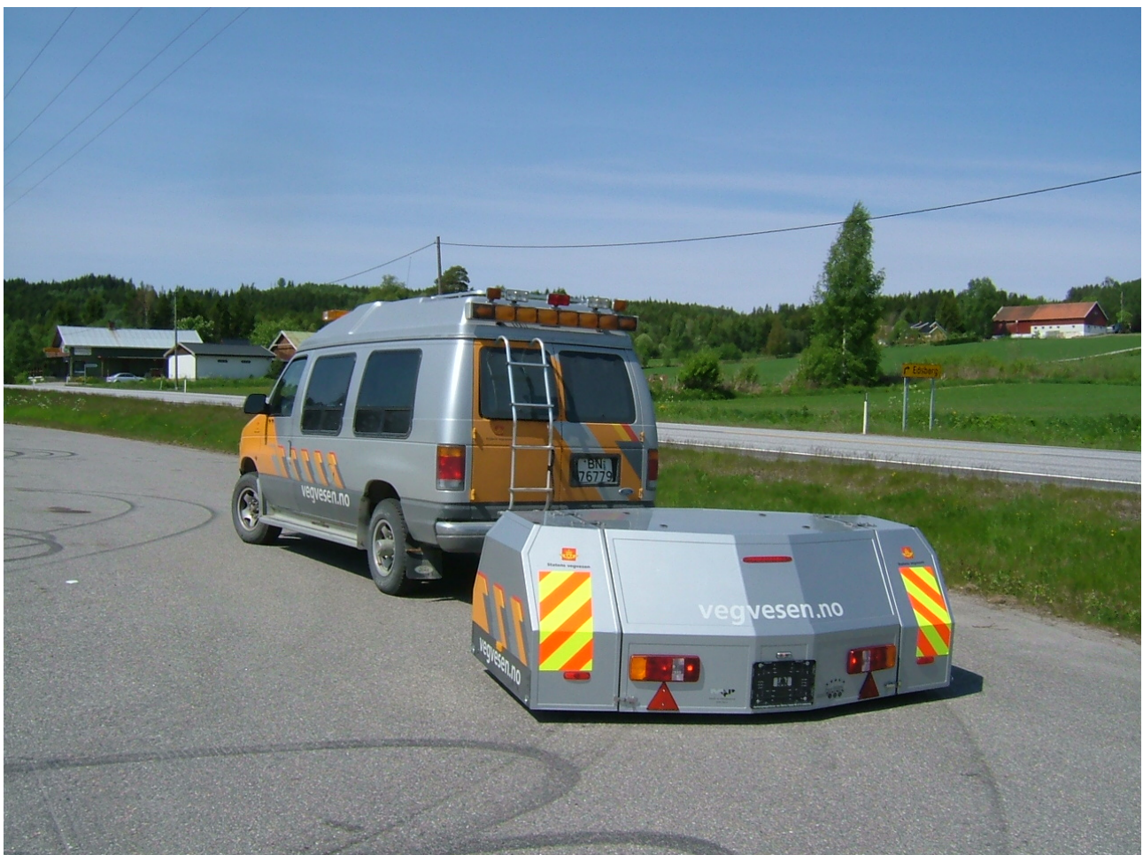
Figure 4.24 The CPX trailer of the Norwegian Public Roads Administration
