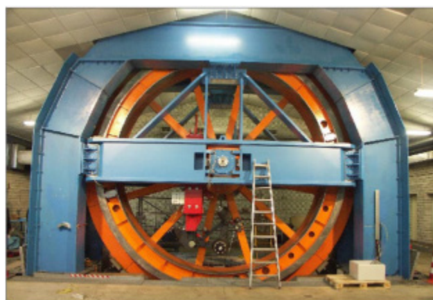
Figure 4.90 The drum facilities at BASt, called PFF (Prüfstand Fahrzeug-Fahrbahn)
