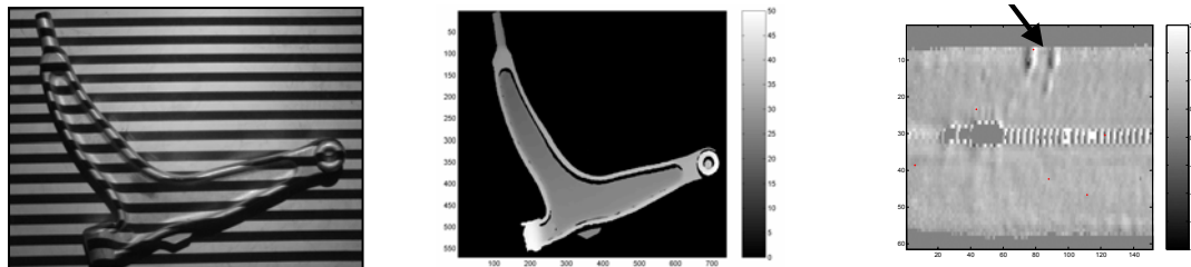
Figure 6: Car part illuminated by structured light (left), obtained 3D model (center) and close-up of two small cracks at the side of the part (right)
