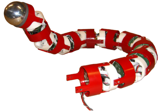
Fig. 1. The NTNU/SINTEF snake robot 'Aiko'.
