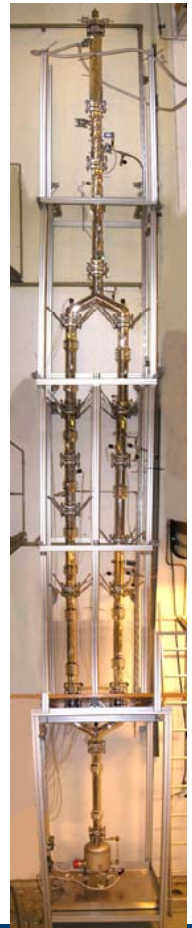
4-product Kaibel-column with a dividing wall
