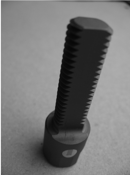
Figure 3: The same bolt as in Figure 1 with a wear resistant DLC coating covering the complete sensor structure except for contacts at the bolts head.
