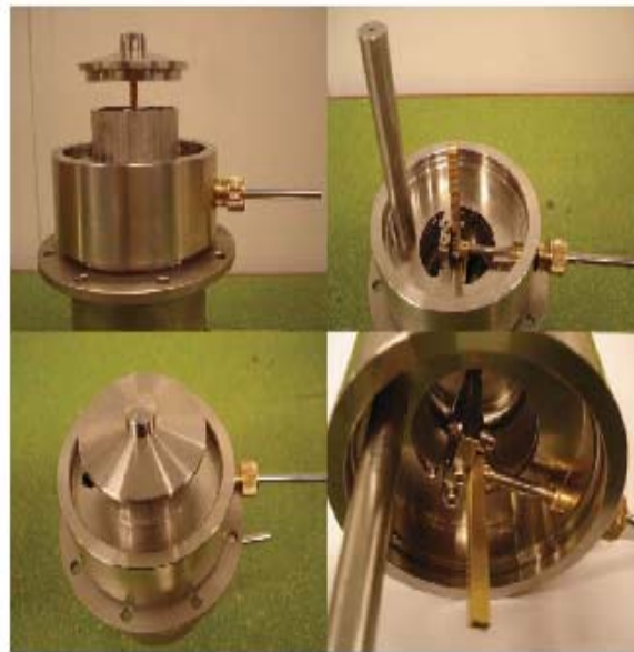
From top left: Valve in fully open position Top right: Rack and pinion arrangement.
