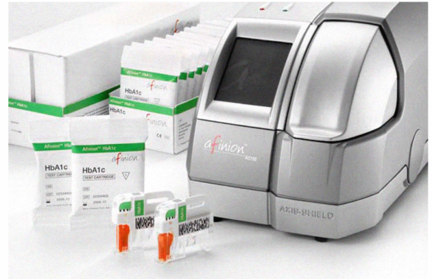
Fig. 1. The Axis-Shield platform Afinion (from www.afinion.net ). Disposable polymer cartridges have all reagents necessary for analysis on-board. The patient blood sample is collected in a capillary tube which is a part of the cartridge. The cartridge is inserted into the instrument and the result can be read out on the display.
