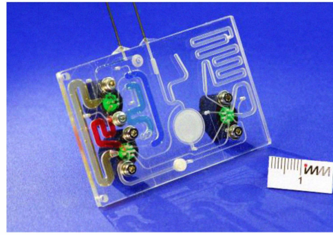
Fig. 3. The MicroActive device accepts 3 ml of sample and performs the extraction in a disposable polymer chip of credit card size. Tests performed using cancer cell lines and cervical liquid based cytology specimens confirm the extraction of HPV-mRNA by the system. Courtesy of IMM.
