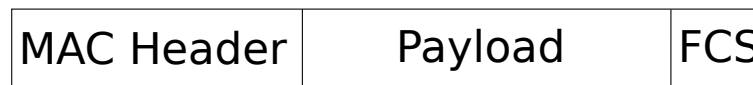
FIGURE 8.2 An 802.11 frame. The MAC header contains the information needed to forward the payload to its recipient, e.g., the sender and receiver MAC addresses. The frame check sequence (FCS) is a cyclic redundancy check used to detect bit errors in the MAC header and payload. If an error is detected, then the frame is discarded.
