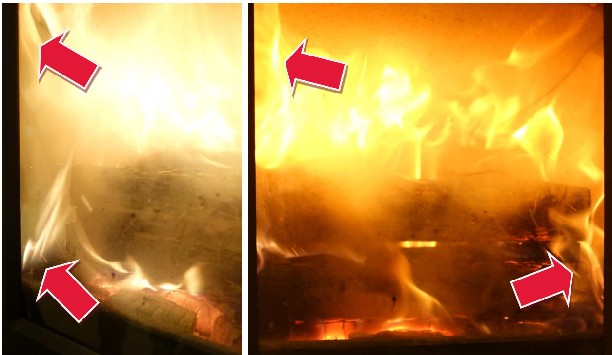
Figure 10: Pictures of test fuel burning in the woodstove burning after removal of door gasket.
