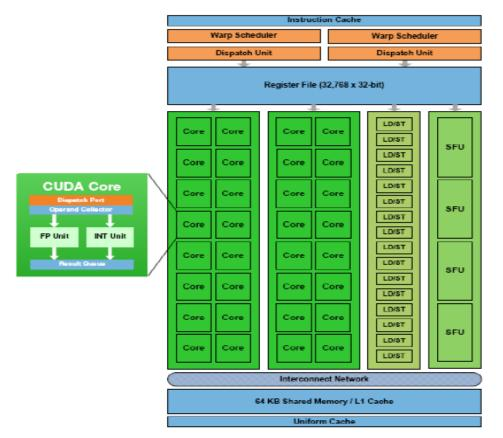
Each of the16 Streaming Multiprocessors (SMs) has 32 cores, 512 cores in total. Each core run the same program («kernel»), with individual data and individual code flow (SPMD). Divergence means serialization. Need more threads than cores to hide latency, typically >512 threads for each SM, say 10.000. One may run multiple kernels concurrently.
