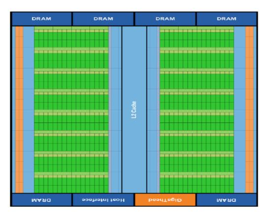
16 streaming multiprocessors are positioned around a common L2 cache
