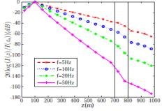
Fig. 1. Current distribution along the wire antenna at different frequencies, f.
