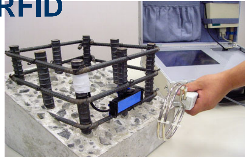
Measures the sensor (white taping area on steel) from RFID tag (in blue) with a portable reader/writer with control PC
