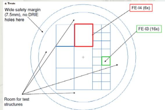
Not final design, FE-I4 chips to be placed symmetrically on wafer
