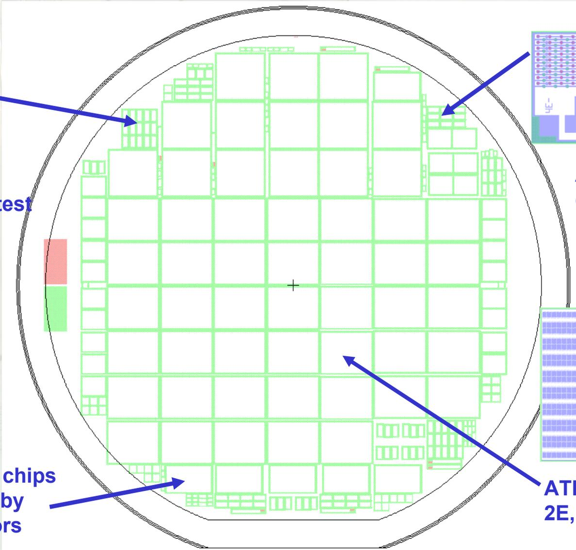
Various test chips including baby strip detectors
