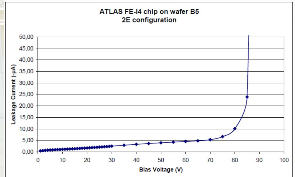
I-V measurements on FE-I4 chips from wafers B2-1, B2-9 (200 µm thick) and B5 (280 µm thick)
