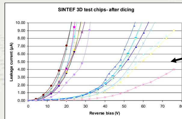
After dicing highly increased leakage
