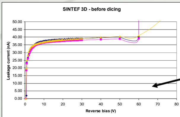
FE-I3 chips total leakage current
