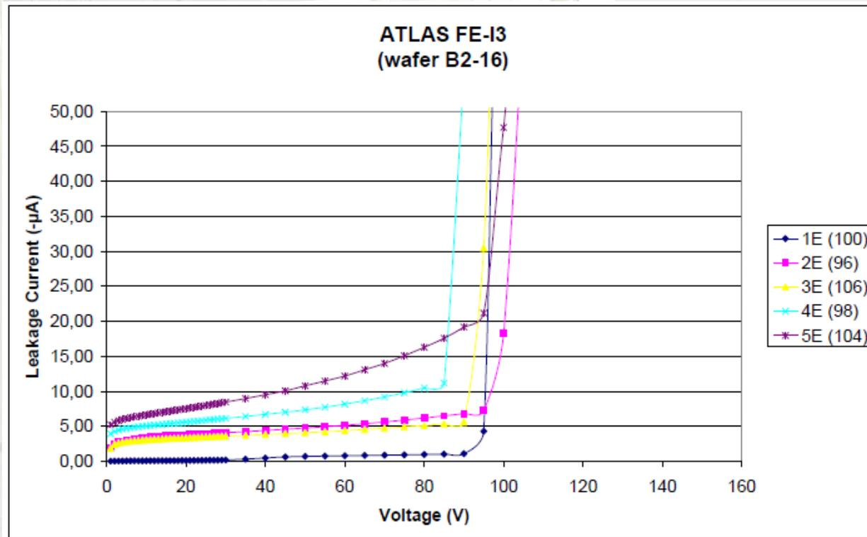
Measured I-V characteristics on FE-I3. Total leakage from  $\approx 2700$  pixels as function of bias. Corresponds to  $\approx 2700$  (1E) to  $\approx 13500$  (5E) electrodes. Leakage includes “MOS” effect and possible bad electrodes.
