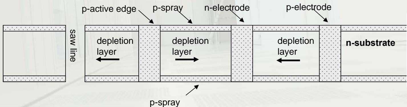
n-readout on n-substrate. oxide and metal not shown
