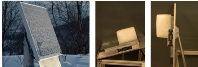
Fig.3. Snow covering a solar cell panel at an inclination angle of 70° (left) and a snow/ice slab strongly adhering to the glass surface of an insulated window pane even at an inclination angle of 90° during a laboratory experiment (right) [13].
