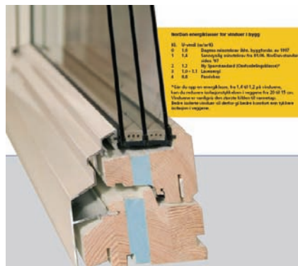
Figure 19. Example of a wood window frame with low U value - N Tech Passiv Superspacer by NorDan AS. Wood frame with PUR. The frame U-value is not stated, whereas the total window U-value is reported to be U_w = 0.7 \text{ W/m}^2\text{K} . From http://www.nordan.no .
