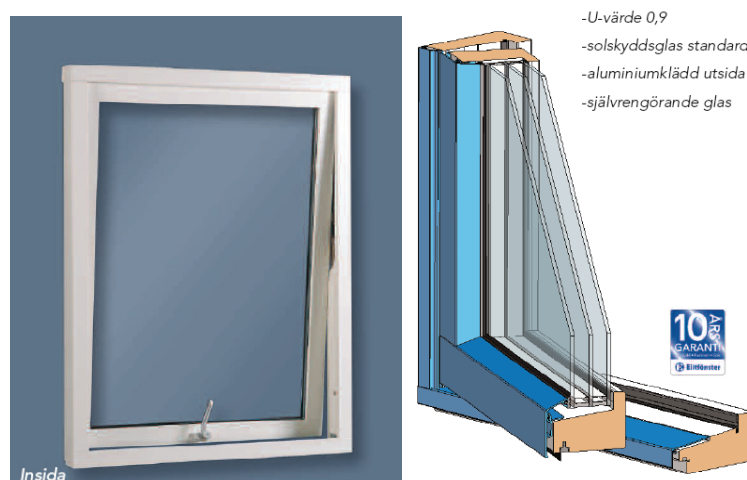
Figure 31. Example of a wood window frame with a relatively low U -value - Elit Extreme 0,9 Fönster, AXH by Elitfönster AB. The frame U -value is not stated, whereas the total window U -value is reported to be U_w = 0.9 \text{ W/m}^2\text{K} . A three-layer window pane is employed in this case with a window glazing U -value of U_g = 0.6 \text{ W/m}^2\text{K} . From http://www.elitfonster.se .
