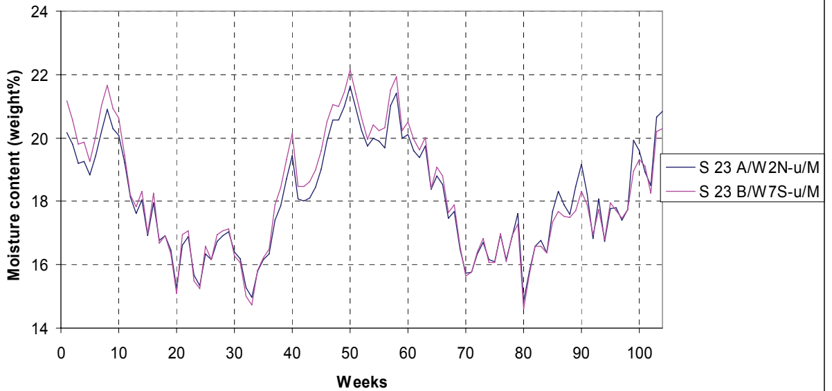
Case 13: Effect of surface treatment (oil, water based) (western orientation, 23 mm air gap, slow growth rate, top of wall)
