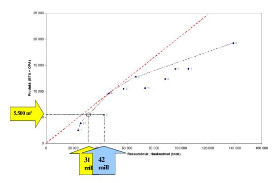
Fig. 5.1 Scatter diagram of Output (Y = Product = BTA + OPA) and Input (X = Resources = Contractor's cost, see figure 2.2) for 11 housing projects
