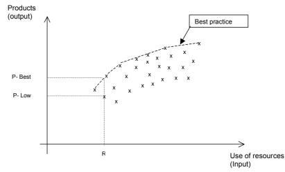
Fig. 4.3 Illustration of the DEA Best practice theory/method; Different number of products (P-Best, respectively P-Low) produced by different producing units (x1, x2 .. x.n) with a fixed input of resources (R)
