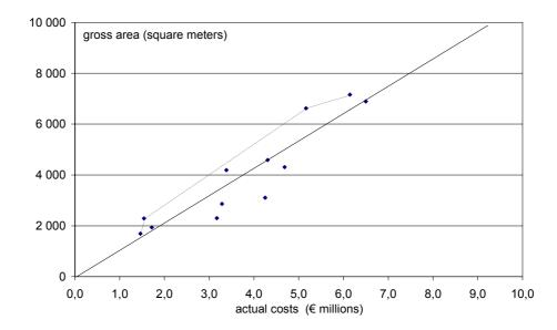
Fig 5.19 Scatter diagram of Output (Y = Product = gross area) and Input (X = Resources = Construction cost) for 12 housing projects. Cost level: year 2003.
