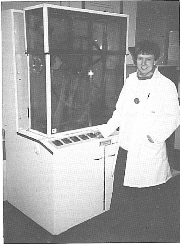
Fig.7. Ozone resistance test equipment
