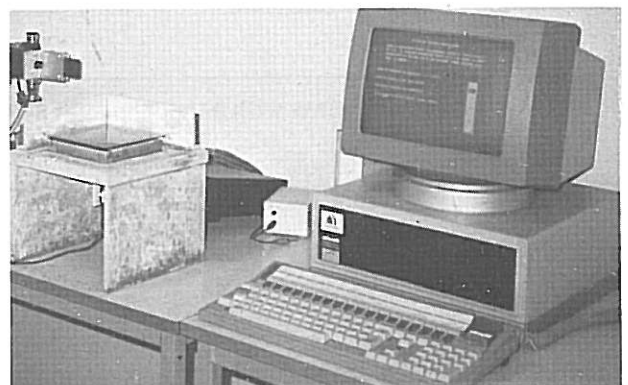
Fig.2. Equipment for testing of deformation resistance
