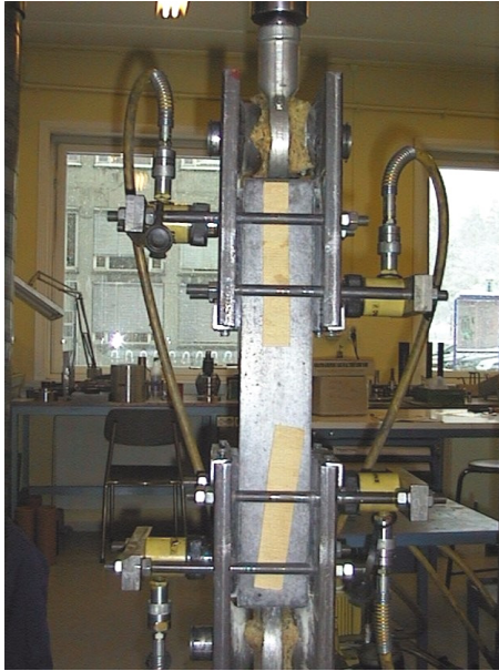
Figure 45 Set-up for testing tensile strength. Uniaxial strength test on prisms (left) and splitting strength test on cubes or cylinders (right)
