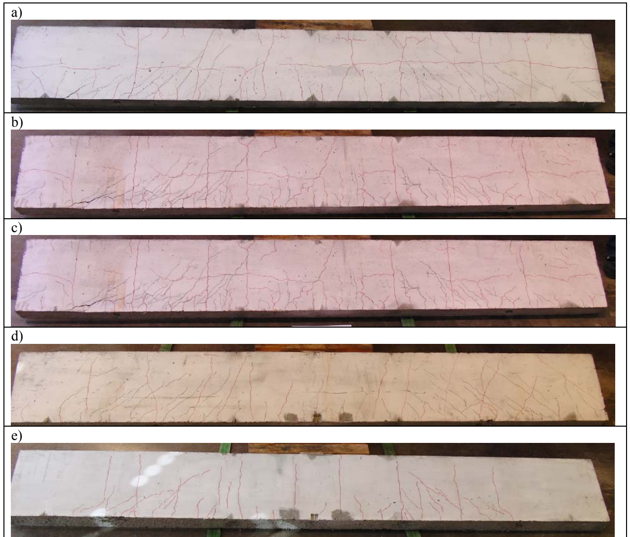
Figure 26. Pictures of composite beams, a) 5C- No fibres, b) 5D -No fibres, c) 9B – 0,5% Barchip synthetic fibres, d) 10B – 0,5% Barchip, e) 7A-0,5% Dramix end hooked steel fibres (65/35).
