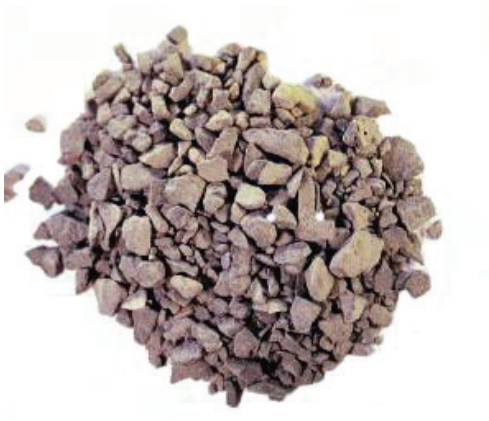
Figure 1-2 Example of crushed, manufactured sand. Particles are in general angular and have broken surfaces
