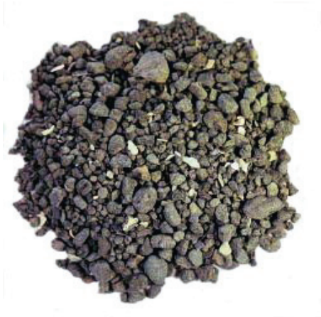
Figure 1-1 Example of natural sand deposit. Particles are in general rounded.
