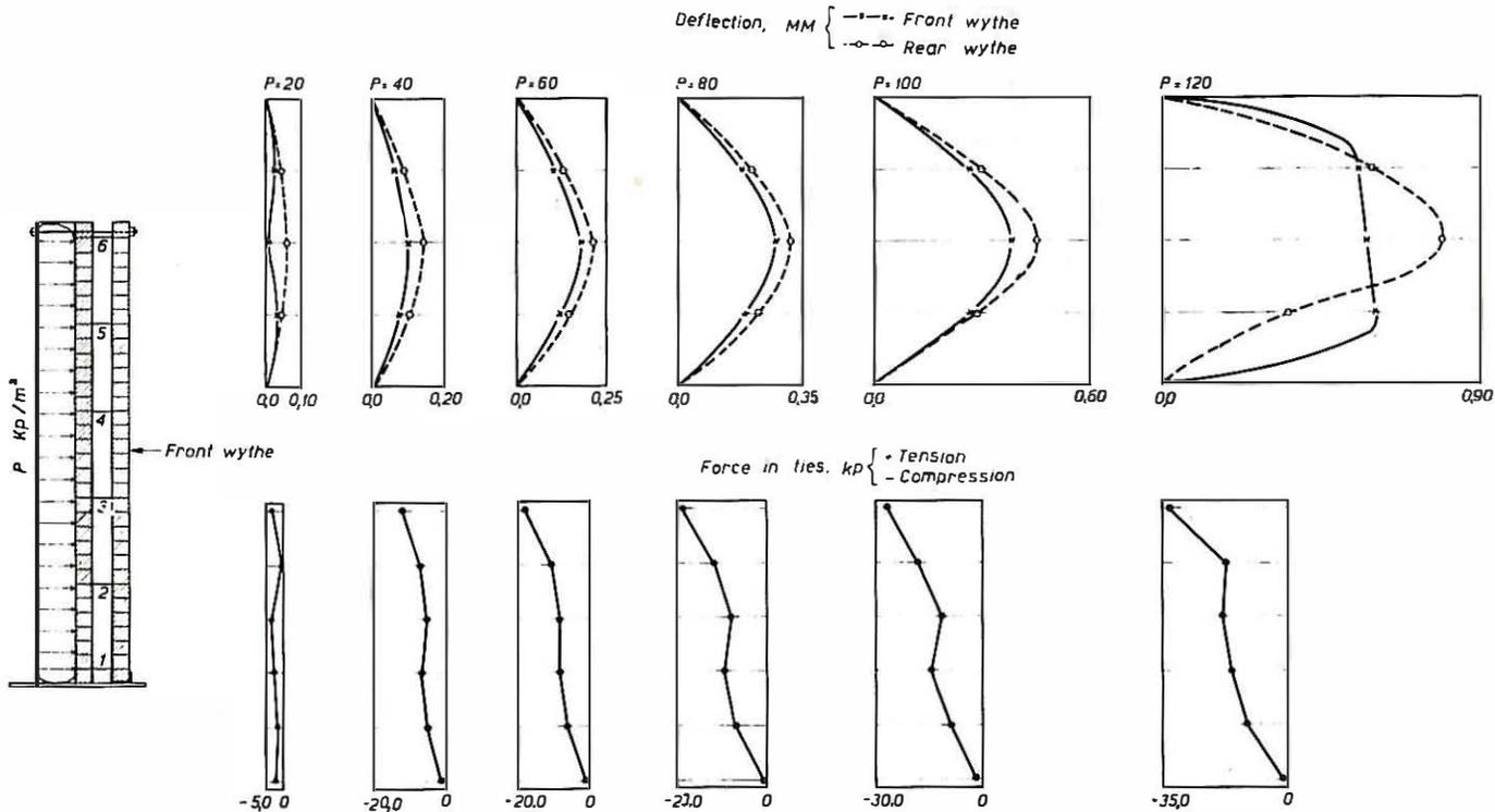
Fig. 4. Test series 1. The curves show measured deflections and the force in the steel ties connecting the wythes, each point on the curves represents the average of 3 measurements.
