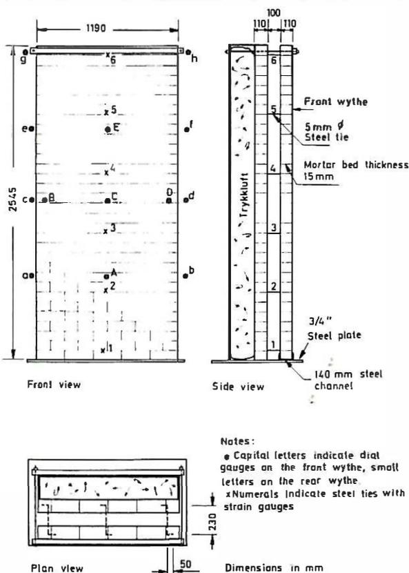
Fig. 1. Dimensions and test arrangement for 1,20 x 2,55 m cavity walls, test series 1.
