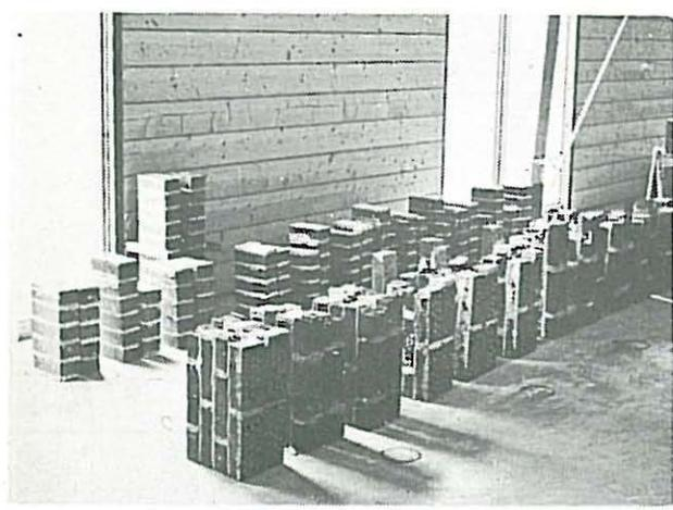
Fig. 3. Piers and small wall panels tested to failure.
