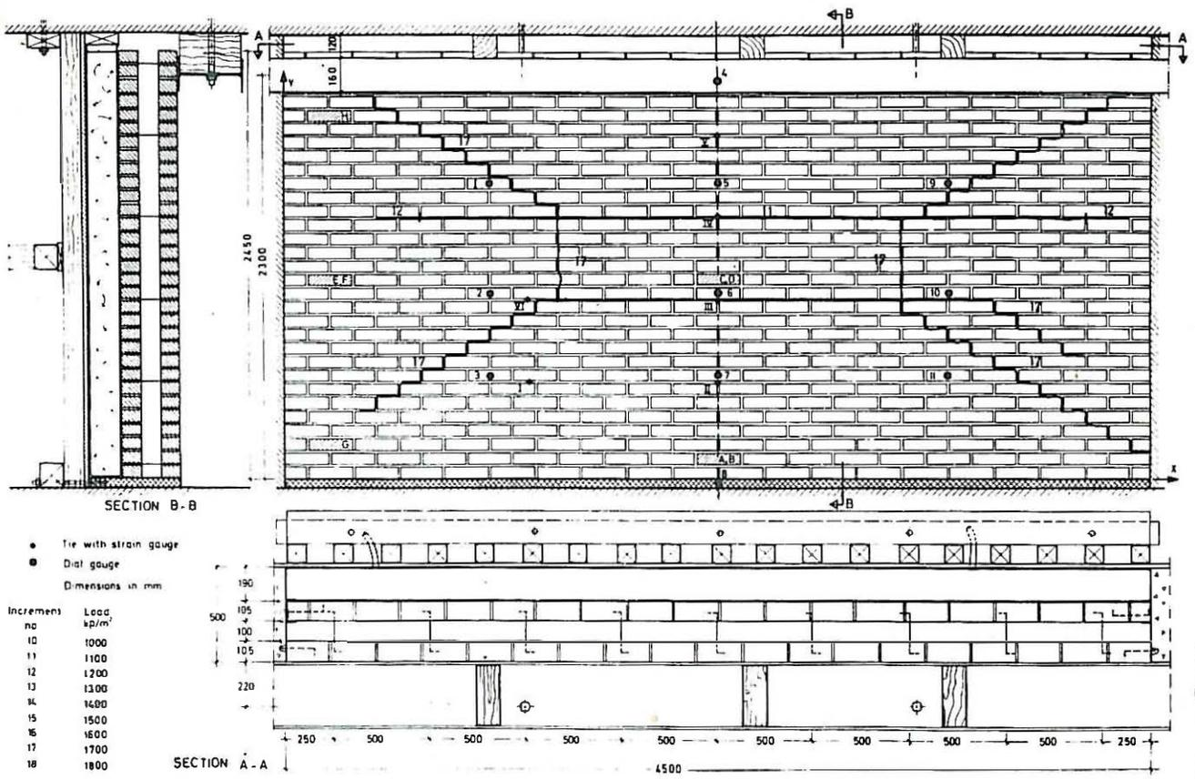
Fig. 2. Dimensions and test arrangement for wall A. The crack pattern is marked on the front wythe.
