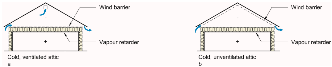
Figure 3. Roof Type C with cold attic. (a) Cold, ventilated attic space with air stream flowing through the attic itself. (b) Cold, unventilated attic space with all ventilation between the underlayer roof and the roof covering. Image further developed from [16].
