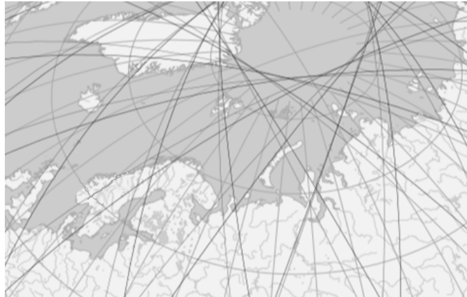
Fig. 1: North Europe view of AISSat1 and AISSat2 orbits over a 24-hour period
