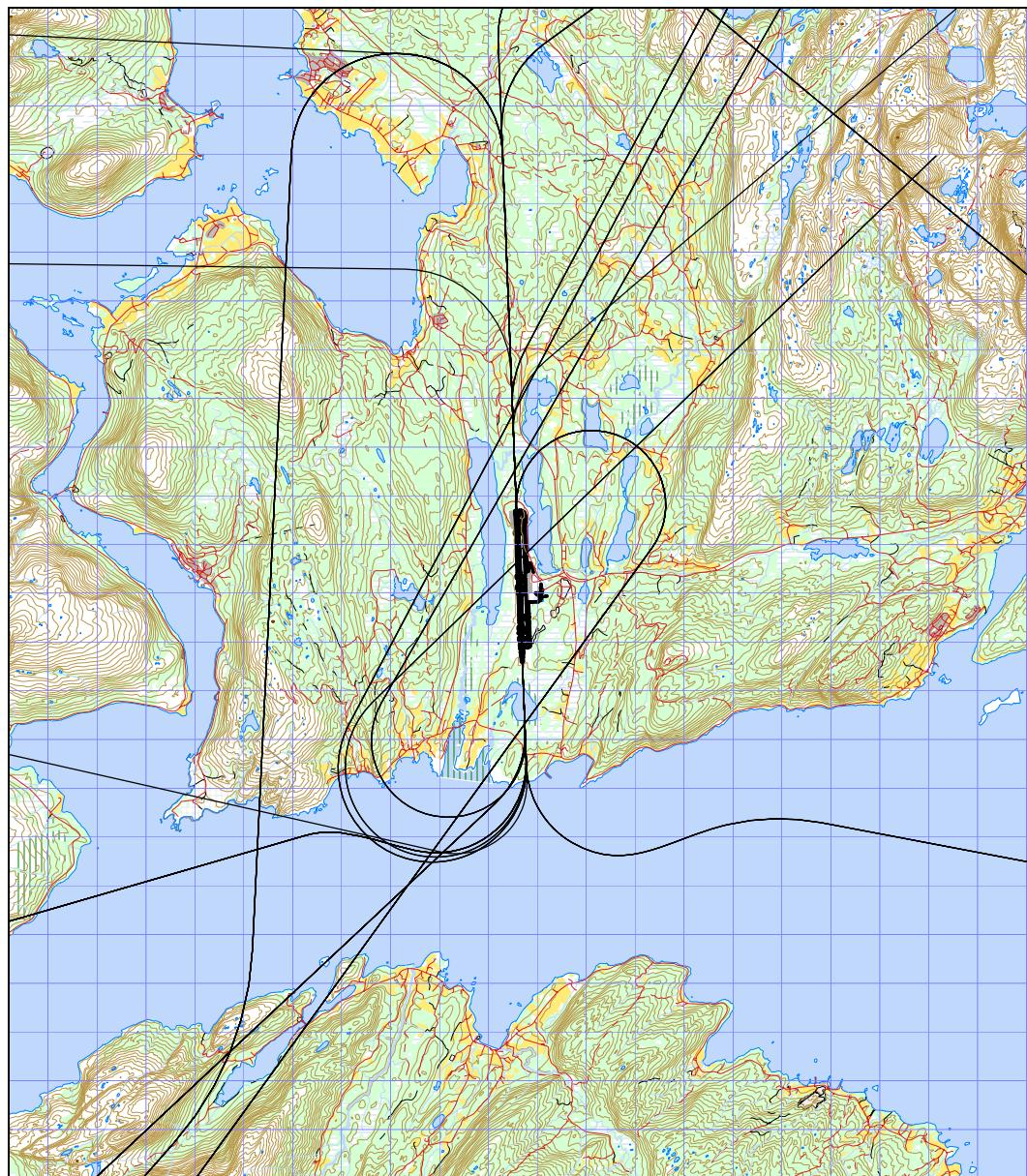
Figur 7-6 Avgangstraséer for jetfly.
