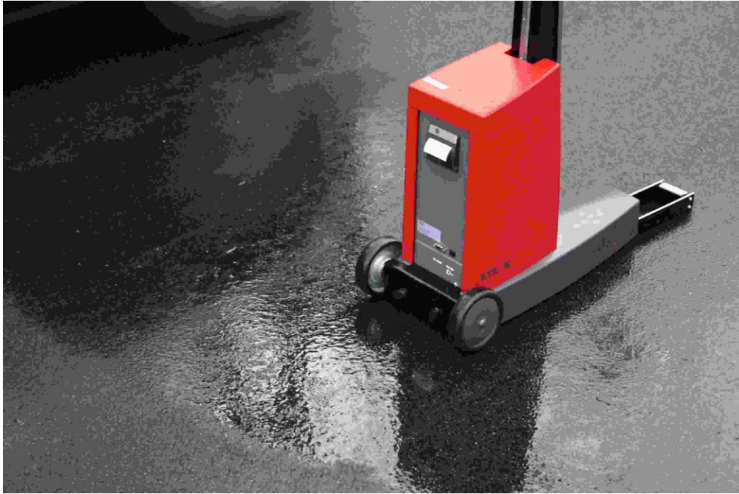
Figure 7.7: A handheld retroreflectometer using the CEN 30 m geometry with modification to provide the specular reflection value instead of the retroreflection value.
