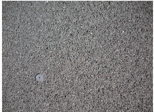
Surface S16: Double layer porous 2/6 + 11/16
