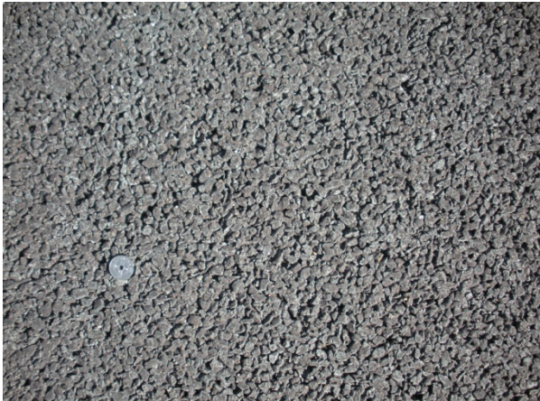
Surface S11: Double layer porous 4/8+11/16
