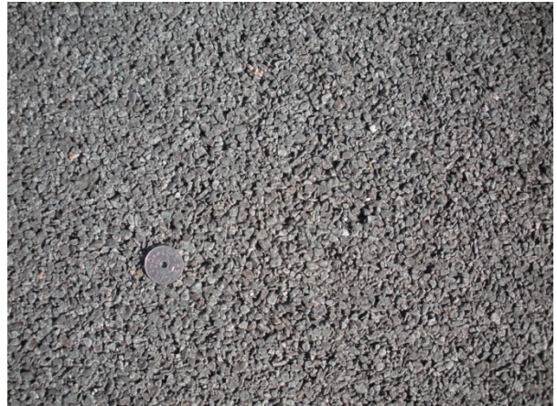
Surface S14: Double layer porous 2/6 + 8/11
