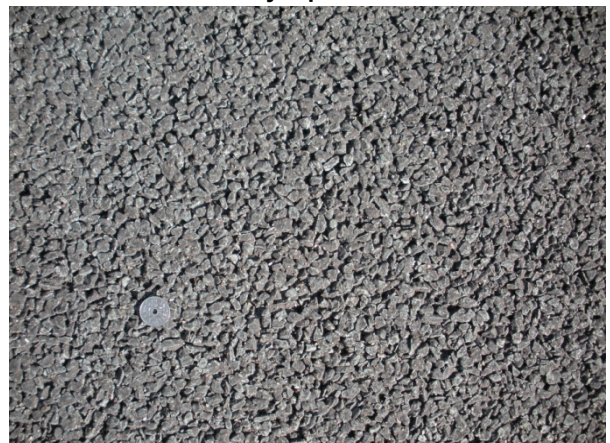
Surface S10: Double layer porous 4/8+11/16
