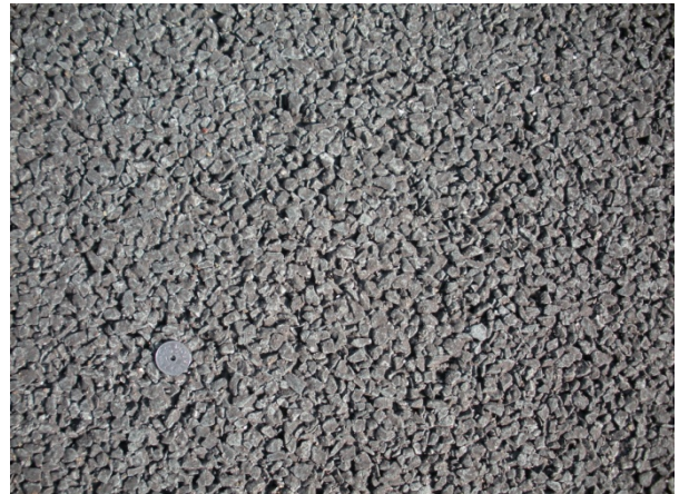
Surface S10: Double layer porous 4/8+11/16
