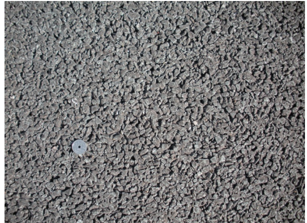
Surface S8: Single layer porous 4/8
