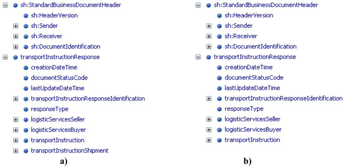
Figure 39 The Transport Instruction message when a) not fully accepted and b) fully accepted
