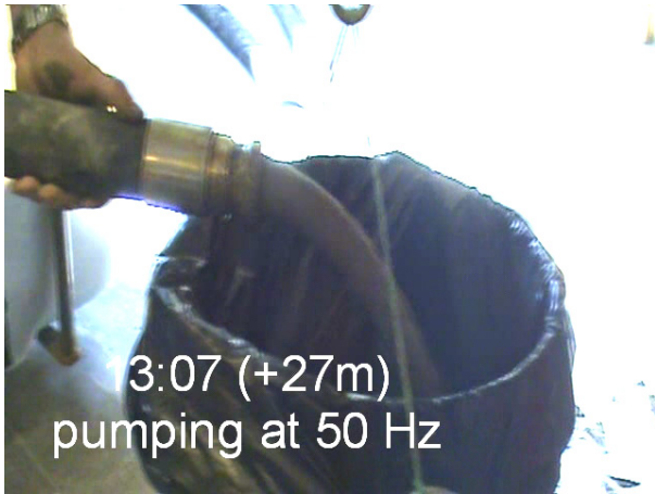
Figure 8: Liquid-like appearance of flow leaving hose end during pump flow measurement
