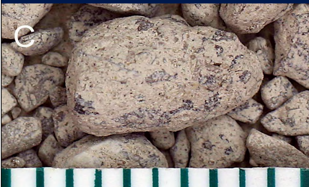
Limestone crushed sand , 11.5 % fines, 2.4 % Absn, 2.554 RD
