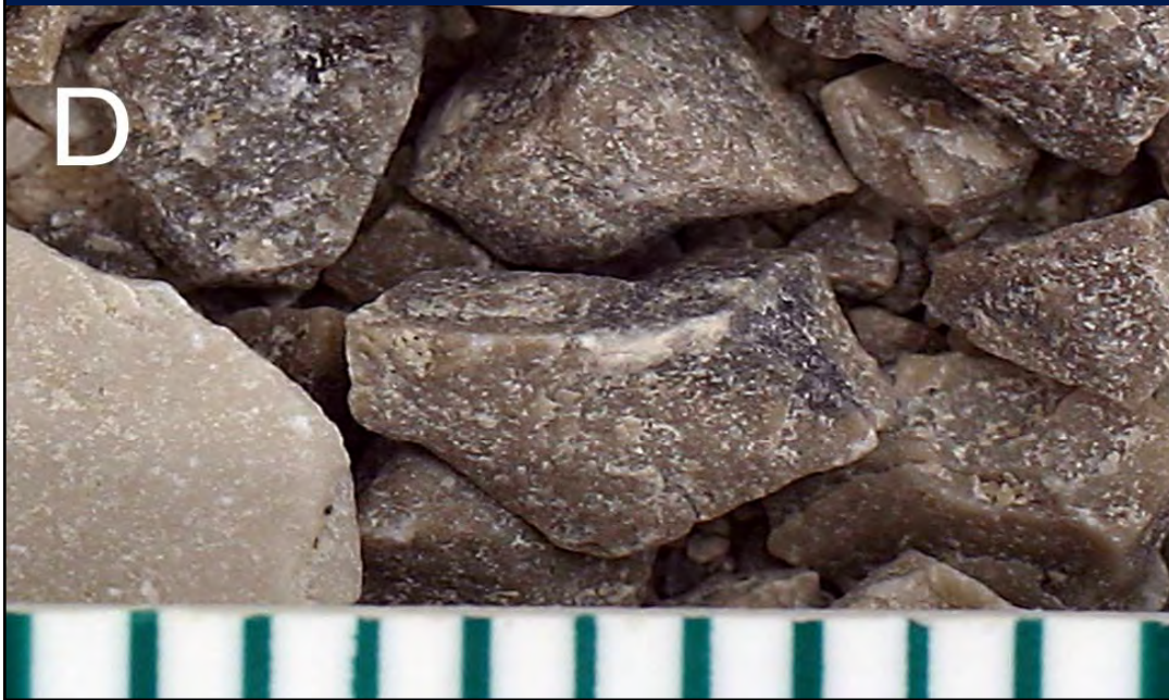
Limestone crushed sand, no fines, 0.74 % Absn, 2.639 RD
