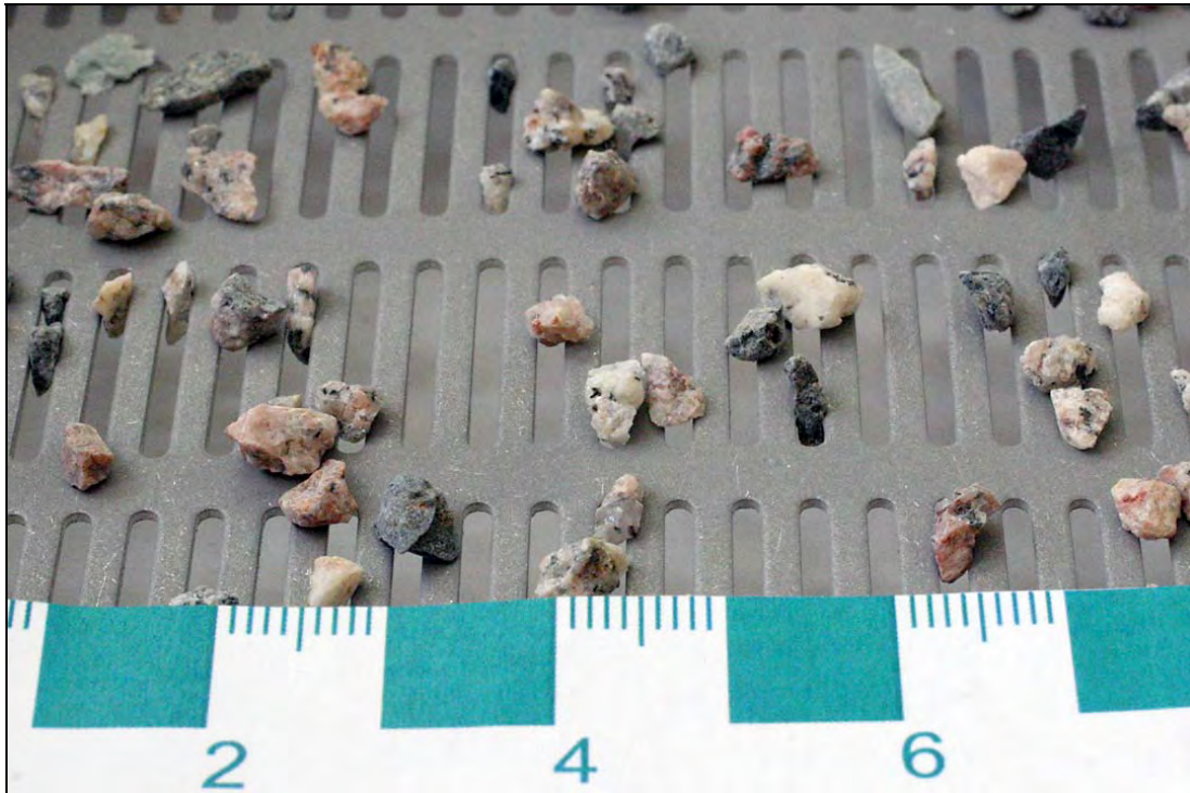
Photo 3 – Aggregate particles retained on the 1.80 mm slotted sieve (Scale in cm).
