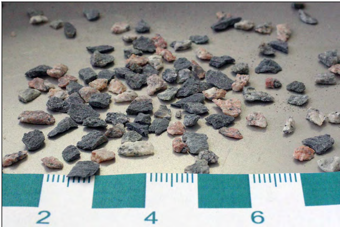
Photo 4 – Flaky particles that passed through the 1.80 mm slots (Scale in cm).
