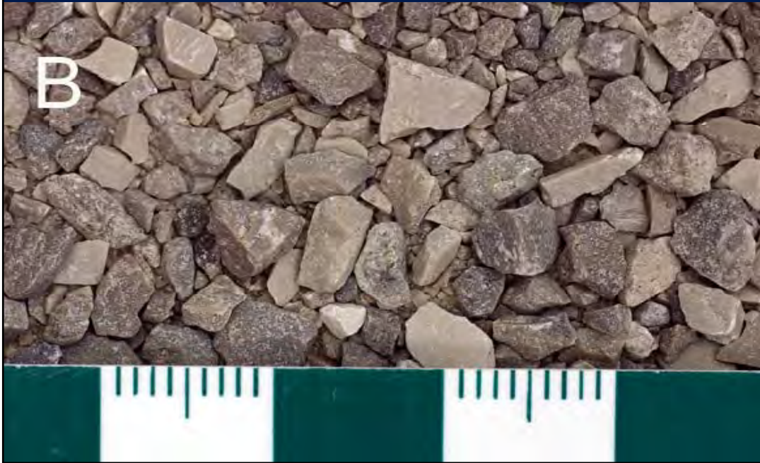
Limestone crushed sand, no fines. 0.74 % Absn, 2.639 RD
