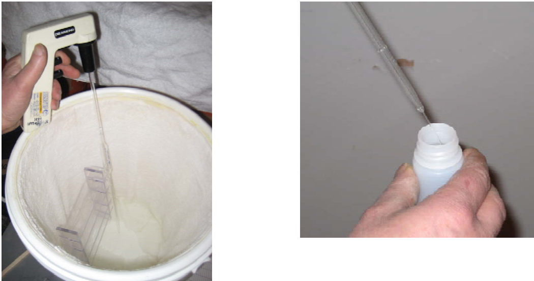
Figure 2. Sampling of water in a container by use of a pipette (left). Plastic bottle for storage of the water sample (right).
