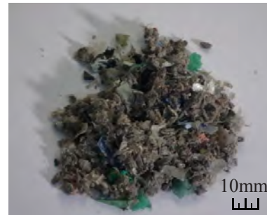
Figure 11: Processed waste plastics for injection into the furnace.
