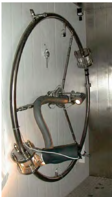
Figure 1: Wheel Flow Loop located at the Tiller Laboratory, SINTEF Norway.
