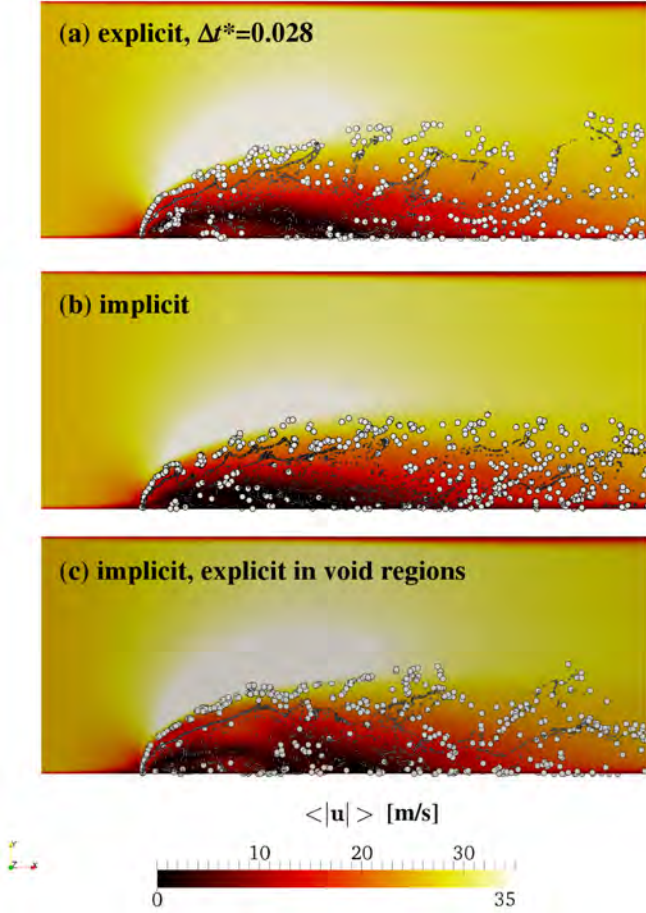
Figure 6: Time-averaged magnitude of the fluid velocity (contours), and particle distribution in the 2D JICF test case ( \Delta t^* = 0.138 ; the simulations in panel c employed impl./expl. force splitting; smoothing based on the local particle diameter was applied; particles are scaled according their primary particle diameter).
