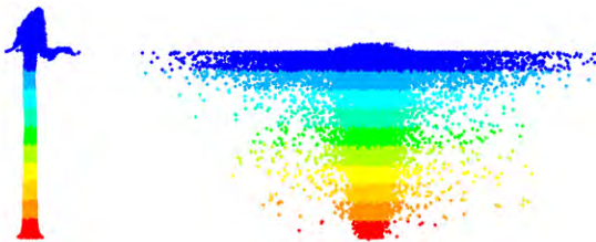
Figure 6: Plume shape coloured by gas density for simulation with neglected (left) and included (right) turbulent dispersion.
